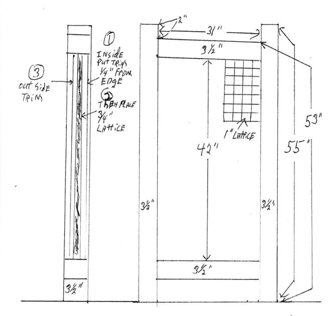
PLACE GAS BOTTLE ON CONCRETE OR CONCRETE BLOCKS. MAKE IT LEVEL BEFORE GAS BOTTLE IS IN PLACE. HOUT 38"X 38" By Russell MAY 2015
